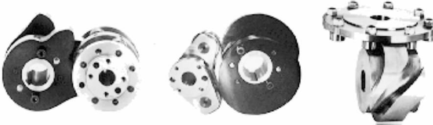
The major feature of the cam drives manufactured by COLOMBO FILIPPETTI consists in the transformation of constant oneway rotary motion from intermittent to simple, direct motion by the use of ground, hardened, conjugate profile steel cams on which at least two cam followers, pre-loaded on assembly, roll simultaneously in opposite directions.
