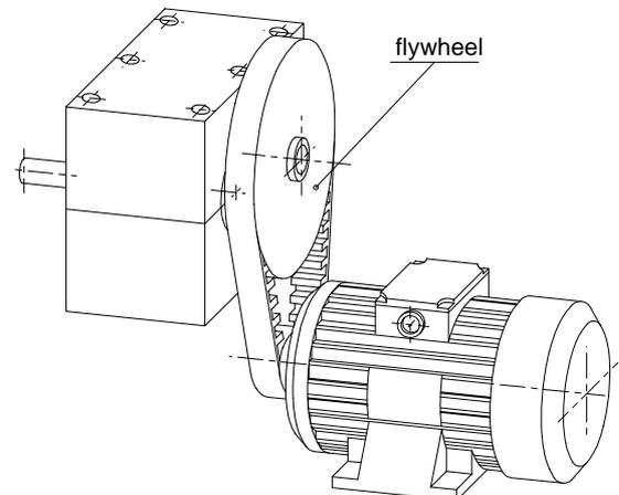
Fig. 8 Motor drive using spring drive; the flywheel ensures that the input shaft rotates at a constant speed.
