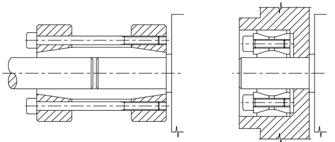
Fig.11 Tapered screw gear spline coupling.
