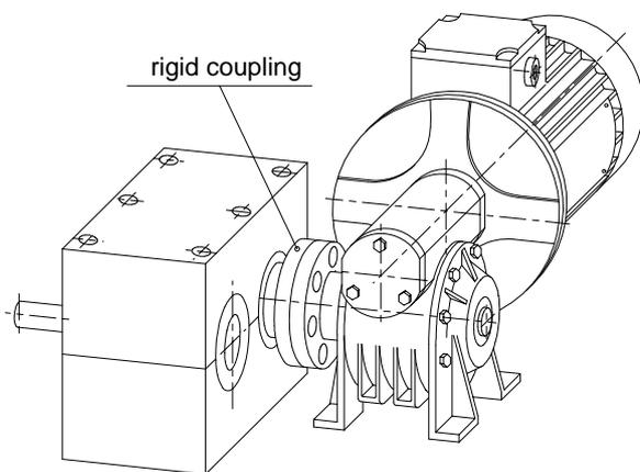
Fig. 7 Motor drive using connection with rigid coupling.
