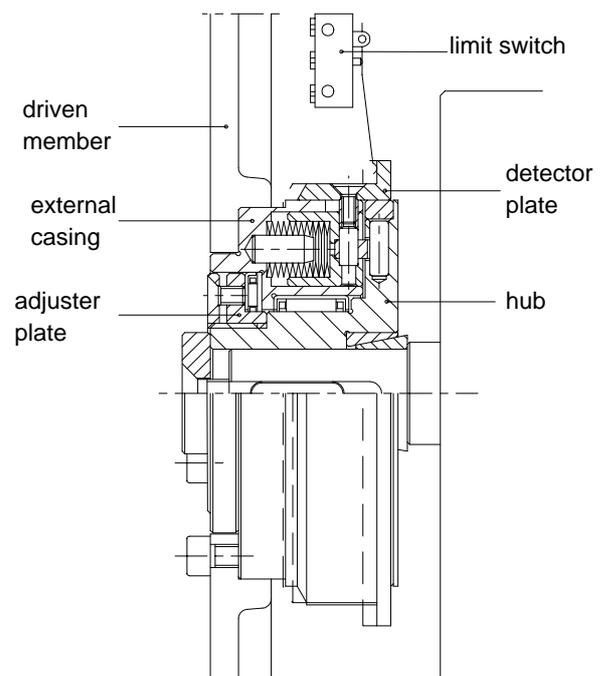
Fig.12 COLMBO FILIPPETTI type GSR output overload clutch.
