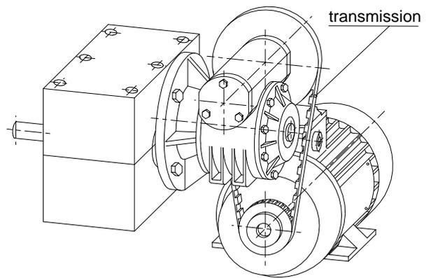
Fig. 6 Rigid motor drive with transmission of fast worm gear reducer shaft.
