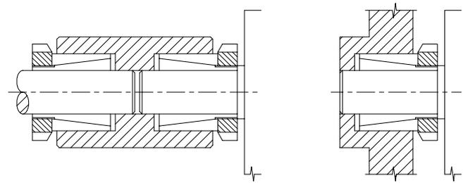
Fig.10 Tapered ring spline coupling.
